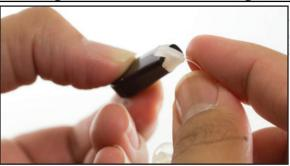
Firmly twist the base of the sound tube until it is perpendicular to the device
